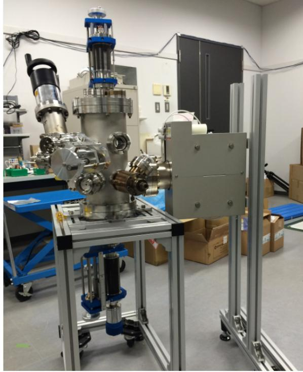
Figure 4.1: The picture of the evaporation chamber. This evaporation chamber is made from SUS 304 chemically polished on the inner surface. The vacuum was maintained with an ion pump (ULVAC PST-100 100 l/s pumping speed)[102] and NEG (Non Evaporative Getter , SAES Capacitorr-D400 480 l/s ) [103] and was kept at UHV (a typical pressure was  $1.0e-8$ Pa).
